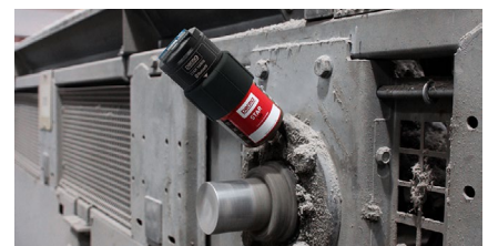
Lubrication of flange bearing on a conveyor
