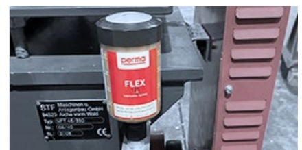
Lubrication of a blower during cleaning
