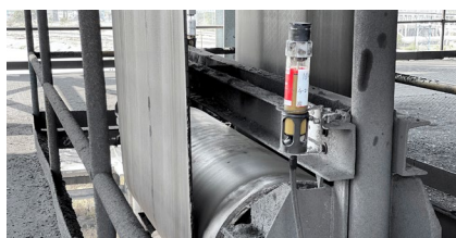
Lubrication of a gravity take-up
