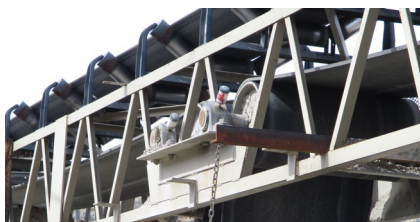
Lubrication of a gravity take-up
